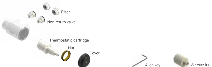
Illustration 5: Exploded view of TMV
