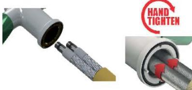
**UK:** Hose connection must be tightened as shown.
